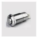
Diameter: Ø 12mm Switch Rating: 2A/36VDC Contact Configuration: 1NO Operation Type: Maintained Lamp type: Ring illuminated (LED) The Crust Material: Stainless steel IP Degree: IP67, IK08
